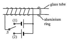
Initially the ring is at rest and the 2-way switch S is in open circuit. In what direction would the ring move at the moment when S is connected in turns to (1) and (2)?
