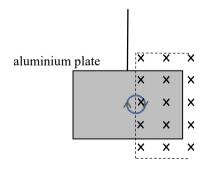
Correct position (accept just within the magnetic field) 1A Correct direction (clockwise) with complete circular path inside the aluminium plate 1A
