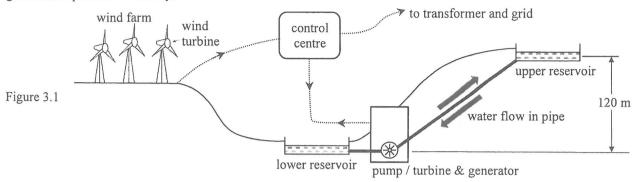
A rotor blade of each wind turbine is 30 m long. Each turbine can be automatically controlled so that the blades' rotational plane is always normal to the wind direction. The graph in Figure 3.2 shows how the electrical power output from each turbine varies with wind speed.
