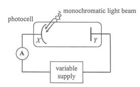
The set-up in Figure 2.1 is for the study of the photoelectric effect. A monochromatic light beam with each photon of energy 3.4 eV is directed towards the photo-sensitive cathode X of a photocell. The potential difference V across anode Y and cathode X can be changed by adjusting the variable supply. The graph shows how the photoelectric current I varies with the potential difference V.
