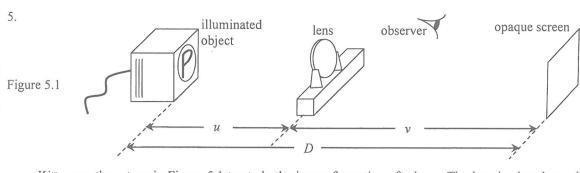
Kitty uses the set-up in Figure 5.1 to study the image formation of a lens. The lens is placed at a distance u from an illuminated object (letter 'P'). An opaque screen is placed at a distance D from the object so as to capture the image.
