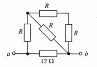
In the above network, the resistance across terminals a and b is 6  $\Omega$ . If the 12  $\Omega$  resistor is replaced by a 6  $\Omega$  resistor, the resistance across terminals a and b
