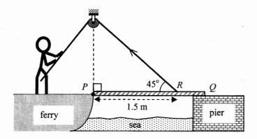
*initial* force required to raise the gangplank when it is horizontal
