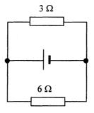
In the above circuit, the cell has e.m.f. 12 V and internal resistance 2  $\Omega$ . What is the current in the 6  $\Omega$  resistor ?
