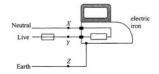
The figure shows a simple domestic circuit for an electric iron. The fuse will blow when which of the following points are short-circuited ?
