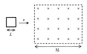
A square metal frame of length of side L moving with constant velocity v passes through a region of uniform magnetic field of width 5L as shown. What is the total time period during which a current is induced in the frame ?
