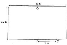
In the above figure, P is a point vertically below the lamp at the ceiling. If the luminous flux given out by the lamp is 1800 lm, what is the illuminance at the point Q?
