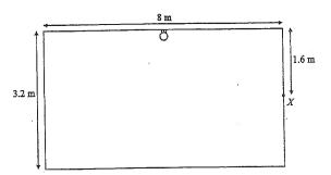
In the above figure, a small lamp given out a total luminous flux of 1350 lm is installed at the middle of the ceiling. What is the illuminance at the point X?
