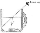
Peter places a coin in an empty cup. As shown in the above Figure, he **cannot** see the coin. After pouring some water into the cup, he finds that he can see the coin without changing the position of the cup or his eyes. In the above Figure, draw a ray diagram to illustrate how Peter can see the coin. (2 marks)
