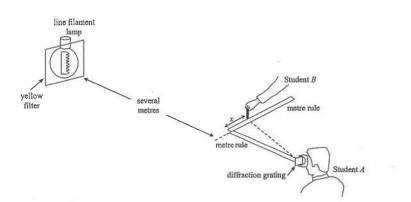
Student A views a line filament lamp with a yellow filter through a diffraction grating with its lines parallel to the filament as shown. The grating is held at one end of a metre rule which is directed towards the lamp. At the other end of the metre rule, a second rule is placed at right angles to the first rule. The diffraction grating has  $6.0 \times 10^5$  lines per metre.
