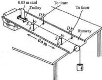
The Figure above shows a trolley running down a friction compensated runway. The trolley is connected to a hanging weight by means of a light inelastic string. A card of width 0.03 m is attached to the trolley. Light sources S and light detectors D are fixed at two positions A and B along the runway. Each light detector is connected to a timer, which can measure the time taken by the card to pass the light detector.
