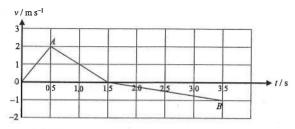
Point A on the graph corresponds to the instant at which the push is removed.
