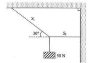
A 50 N block is suspended by two threads as shown in the figure above. Thread  $S_1$  makes an angle 30° with the horizontal and thread  $S_2$  is horizontal. What is the tension in  $S_2$ ?
