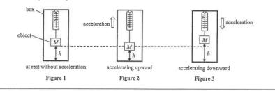
(a) Draw a labelled free-body diagram in the space provided below showing the forces acting on the object when the box accelerates upward with acceleration a. Explain why h decreases in this case.
