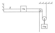
The system of pulleys and blocks is at rest. What is the tension in string S? (Neglect all friction and the masses of the strings and pulleys.)
