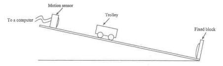
The trolley is released from rest so that it runs downwards along the runway. At the end of the runway, there is a fixed block used to stop the trolley. The velocity-time graph captured by the motion sensor is shown in the figure below.
