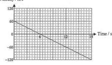
The above figure shows a man near the edge of a cliff projecting a stone vertically upwards. The stone reaches the sea after 18 s. The graph shows the velocity  $\sim$  time for the motion of the stone. Find the height of the cliff. (Take  $g = 10 \text{ m s}^{-2}$ .)
