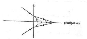
Referring to the above ray diagram, what kind of lens is represented by L? Which point, P or Q, can be its focus?
