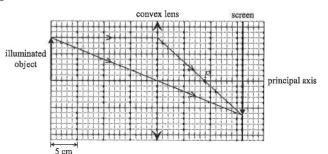
From the above figure, the focal length is about 9 cm, i.e. between 8 cm and 10 cm.
