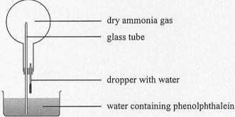
The round-bottomed flask was initially full of dry ammonia gas. Several drops of water were injected into the flask from the dropper. The water containing phenolphthalein was then automatically sucked into the flask through the glass tube.
