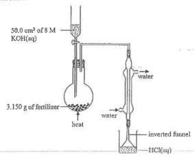
The KOH(aq) was added slowly to the fertilizer and the mixture formed was heated gently. The ammonia liberated from the reaction between NH<sub>4</sub>NO<sub>3</sub> and KOH was first cooled in a condenser, and then passed through an inverted funnel to a solution containing 0.0485 mol of HCl. The solution was finally made up to 100.00 cm<sup>3</sup> and labelled as 'S'.
