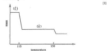
(I mark for showing two 'steps' in the curve; I mark for showing that the heights of two 'steps' are in 4: 1 ratio.)
