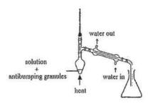
(1 mark for a workable set-up; 0.5 mark for labeling the reagents and 0.5 mark for the direction of water flow in the condenser.)
