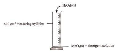
When 10.0 cm<sup>3</sup> of 3.00 M H<sub>2</sub>O<sub>2</sub>(aq) was mixed with a small amount of MnO<sub>2</sub>(s) and detergent solution at room conditions, O<sub>2</sub>(g) started to be released rapidly and foam was produced. The MnO<sub>2</sub>(s) remained chemically unchanged at the end of the reaction.
