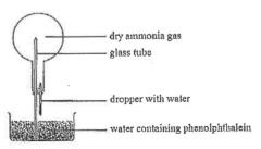
The round-bottomed flask was initially full of dry ammonia gas. Several drops of water were injected into the flask from the dropper. The water containing phenolphthalein was then automatically sucked into the flask through the glass tube.
