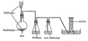
Point out two mistakes in the above set-up, and suggest the corresponding rectifications.
