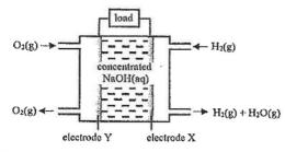
Hydrogen and oxygen are passed into the fuel cell. The half equations for the chemical changes occurring at electrode X and electrode Y are listed below:
