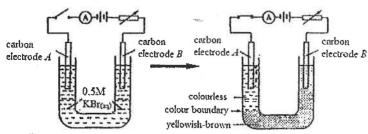
Diagram I: before electrolysis Diagram II: after electrolysing for some time
