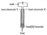
When the lead(II) bromide becomes molten, the bulb lights up,
