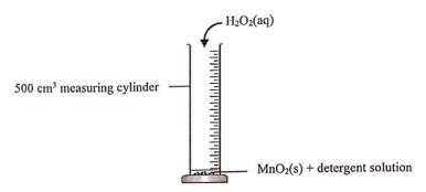
When  $10.0~\rm cm^3$  of  $3.00~\rm M~H_2O_2(aq)$  was mixed with a small amount of MnO<sub>2</sub>(s) and detergent solution at room conditions, O<sub>2</sub>(g) started to be released rapidly and foam was produced. The MnO<sub>2</sub>(s) remained chemically unchanged at the end of the reaction.
