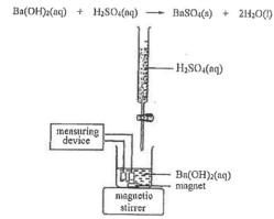
(a) What physical parameter of the reaction mixture is measured by this set-up?
