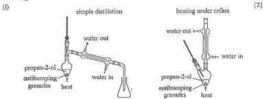
(1 M for a correct set-up and showing the bulb of the thermometer is slightly above the liquid level, 1 M for labels)
